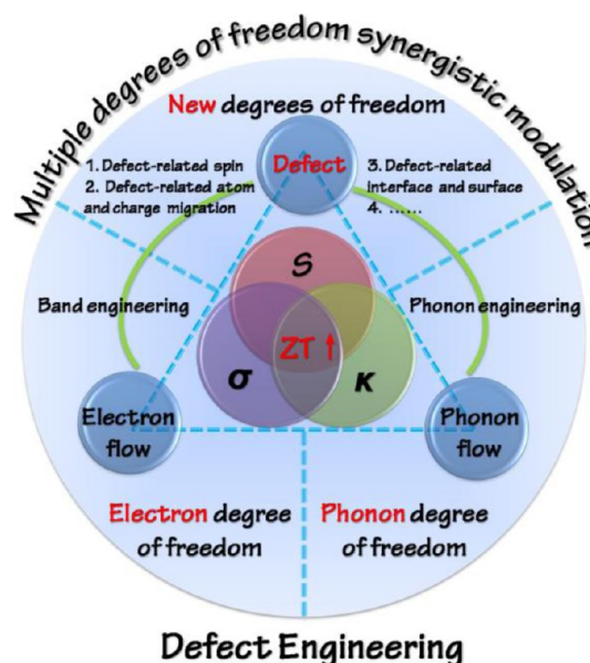
Figure 1. Schematic illustration of the ZT optimization strategies based on defect engineering from the perspective of multiple degrees of freedom synergistic modulation.
